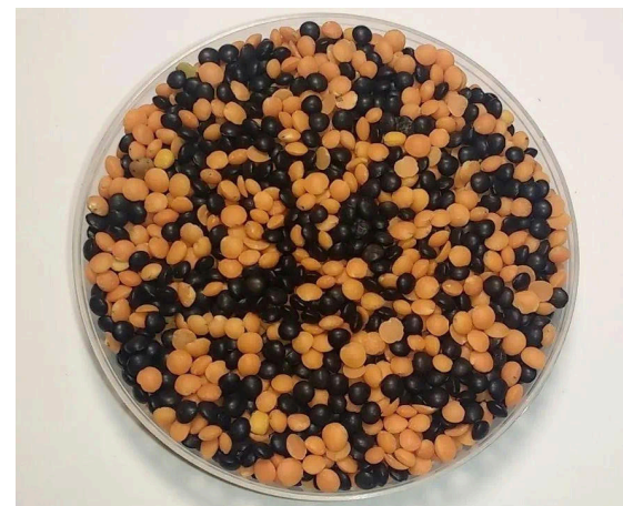
A mixture of red and black lentils with a complex pattern. Electronic devices can be immersed in the mixture so that when they are accessed, the pattern changes.
