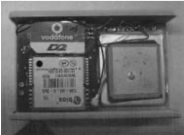
Inside view of a GPS tracking module. At the top left the GSM card for transferring data via cellular network.
