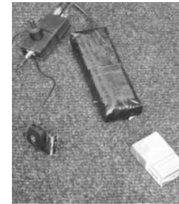
Left: GPS transmitter from the LKA Schleswig-Holstein (2007), GPS antenna and battery set separately.
