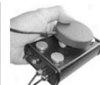
Right: GPS transmitter from the BKA (2007), GPS antenna separately.
