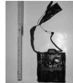
Left: GPS transmitter from the LKA Schleswig-Holstein (2007), GPS antenna and battery set separately.
