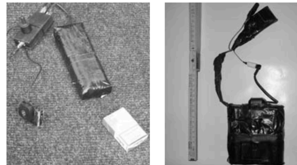
Left: GPS transmitter from the LKA Schleswig-Holstein (2007), GPS antenna and battery set separately.
