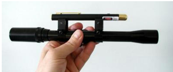
Simple laser / rifle scope system.
