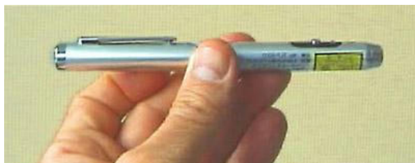
Inexpensive laser pointer (1 mW, 650 nm red).
